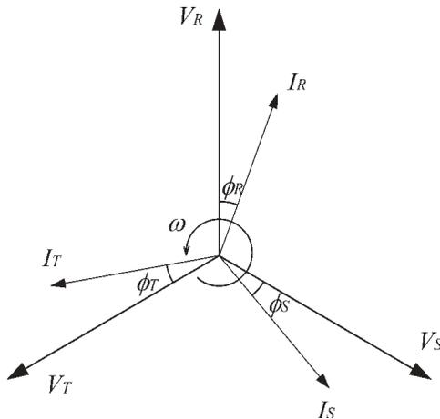
Figure 1. Phasors  $V$ - $I$  diagram.
