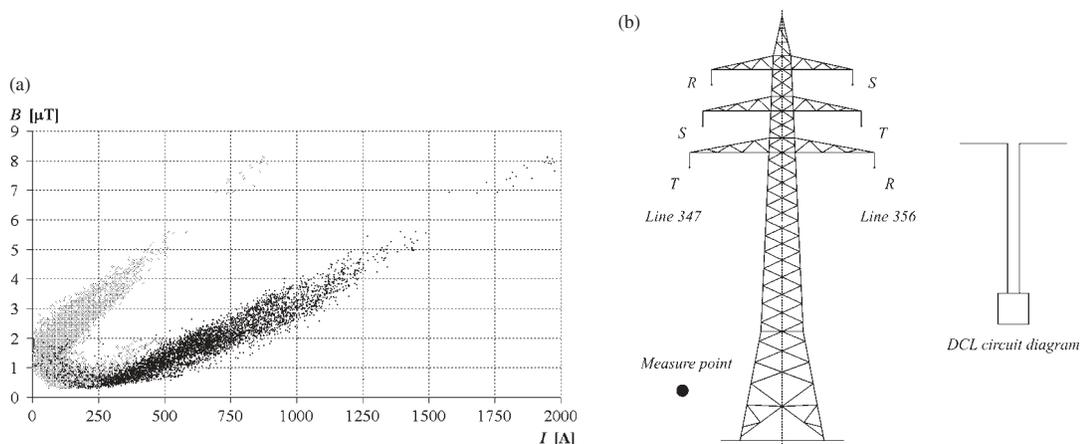
Figure 6. (a) Magnetic induction in function of current for lines 347 (light dots) and 356 (dark dots). (b) Disposition of the phases on a pylon of the 347–356 DCL and relative circuit diagram.
