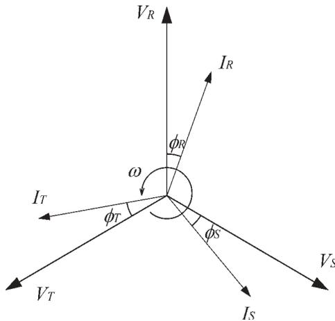
Figure 1. Phasors  $V$ - $I$  diagram.
