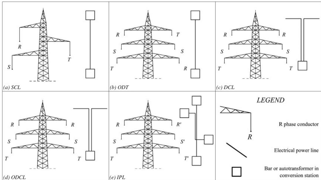
Figure 3. (a–e) Schematic representation of power line typologies.
