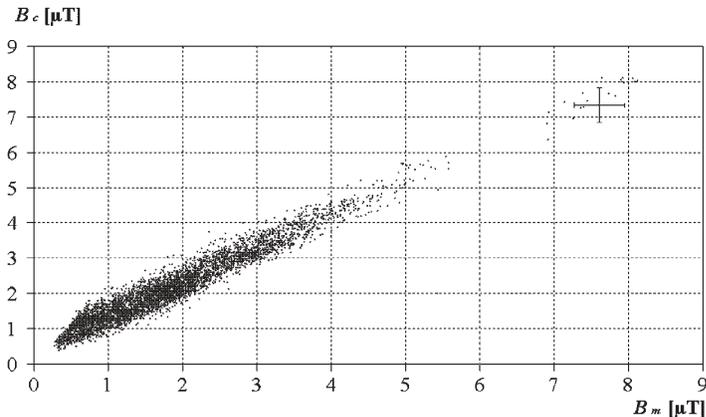
Figure 5. Relationship between induction measured ( $B_m$ ) in proximity to a double line and that calculated by Phidel<sup>®</sup> ( $B_c$ ).
