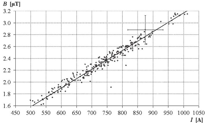
Figure 4. Relationship between measured induction and line current for a single line case (n. 356, 380 kV).
