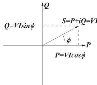
Figure 2. Scalar  $P$ - $Q$  diagram.
